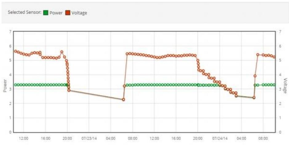
This node has one or more poor or obstructed solar panels, and is repeatedly sleeping, recharging and waking during the day. You can see when the light fades and proper sleeping commences, it's a nice regular slope.
