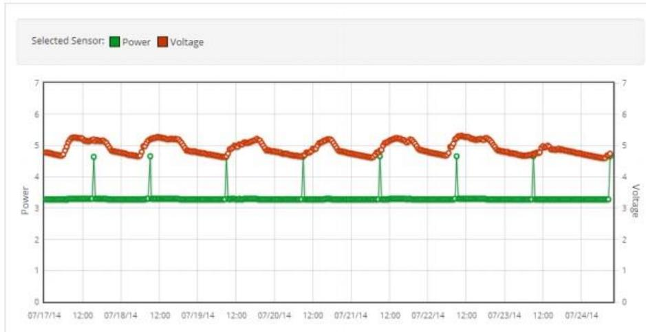
If you see your Base (as below) showing the part of the graph on the left side, or the graph does not even show the vertical dots, it is disconnected from its power storage. If you are seeing the shape on the right, the Base likely has no routing nodes with it or in sight, and so does not know how to sleep.
