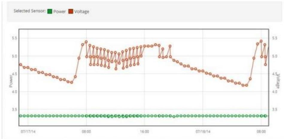
This node is showing normal wake and sleep patterns – the dip at noon shows that neither solar panel is pointed at the light, so it sunny. When there is no dip, it is cloudy because clouds provide light coming from all directions. The spikes indicate the code version: hover your mouse over and divide the reading by two to get this device’s code version.
