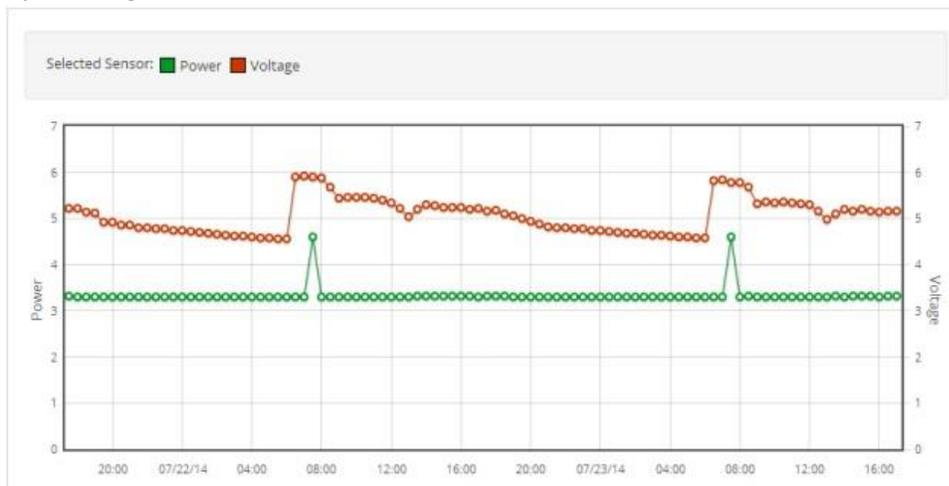
This PC-link or modem gateway’s fuzzy and irregular power supply chart is poor-contact your supplier as there is something wrong with this device and so this mesh will not work as well as it could.
